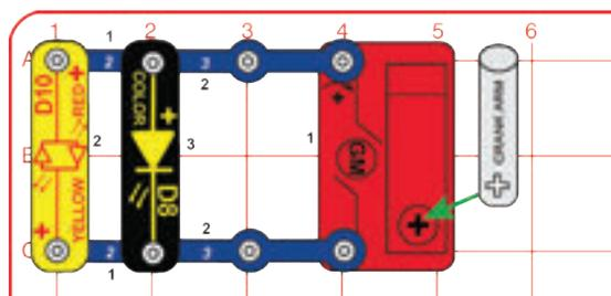
Turn the crank arm clockwise to light the LEDs (D8 & D10). Turn the crank at a constant speed so both LEDs light, and notice how only the color LED is flashing now.
