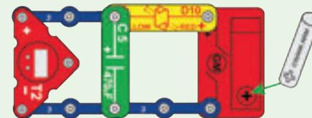
9. **Pivot stand resistors:** The pivot stand base has resistors mounted inside; they can be tested using this circuit. Set the switcher (S6) to the left position and turn the crank arm clockwise; the red/yellow LED (D10) should be bright red. Next, set the switcher to the right position and turn the crank arm clockwise; the color LED (D8) should be on but dim.
