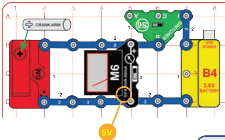
Modify the preceding circuit into this one. Set the meter (M6) to the 5V setting. Set the switcher (S6) to the right position and watch the voltage on the meter when the crank arm spins.
