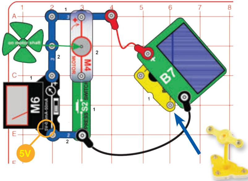
Mount the solar cell (B7) on the pivot stand as shown, and place it in sunlight or near an incandescent lamp. The meter (M6) measures the voltage produced.
