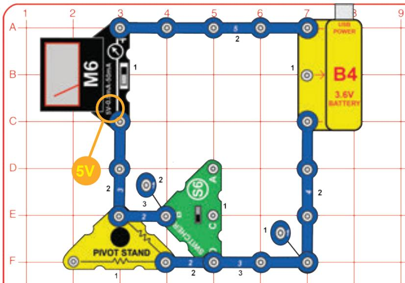
To make a voltage measurement, the meter (M6) is set to 5V and connected in parallel between the two points where the measurement is to be made. Since the voltmeter is in parallel and has a high resistance, very low current flows through it.
