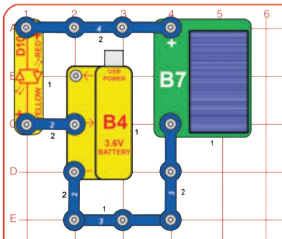
This circuit uses the solar cell (B7) to charge the rechargeable battery (B4). Place the solar cell in sunlight or near an incandescent light bulb. The red/yellow LED (D10) lights red when the battery is being charged. The brighter the LED, the faster it is charging.
