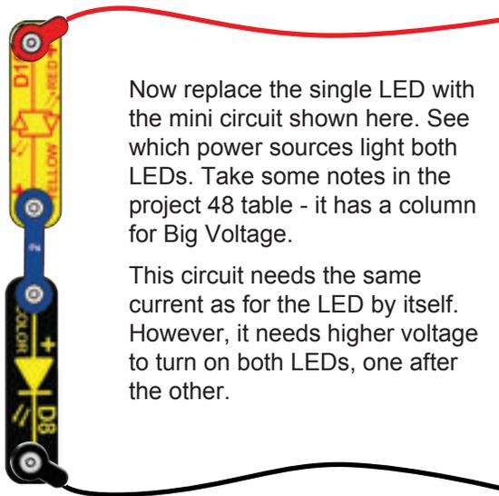
Now replace the single LED with the mini circuit shown here. See which power sources light both LEDs. Take some notes in the project 48 table - it has a column for Big Voltage.
