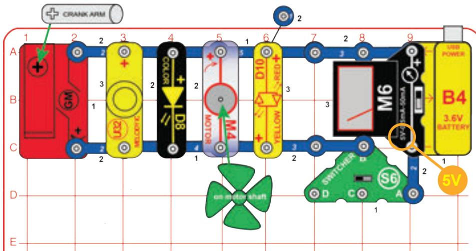
Build the circuit and set the meter (M6) to the 5V setting. Set the switcher (S6) to the left or middle position (off) and read the battery (B4) voltage when it is not running anything.
