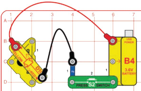
Build the circuit as shown, with the red/yellow LED (D10) on the pivot. Point the LED towards your friends and push the switch (S2) several times to send messages to your friends using Morse Code.
