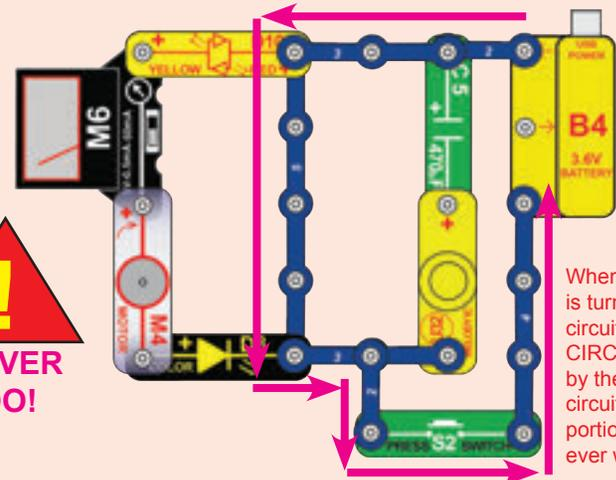
When the switch (S2) is turned on, this large circuit has a SHORT CIRCUIT path (as shown by the arrows). The short circuit prevents any other portions of the circuit from ever working.
