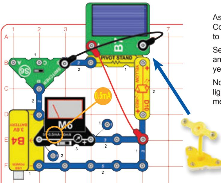
Assemble the pivot, mount the solar cell (B7) on it, and place it in the circuit as shown. Connect the solar cell to the circuit using the red and black jumper wires. Set the meter (M6) to the 0.5mA setting.
