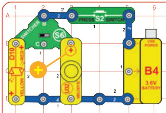
Build the circuit shown and push the press switch (S2) to turn on light or sound. Switches can be arranged in many different ways.
