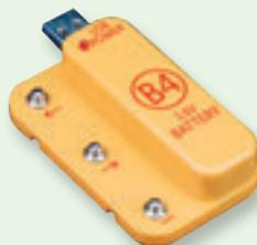
The **battery (B4)** contains a rechargeable battery and some supporting parts. This battery produces an electrical **voltage** using a reversible chemical reaction. This "voltage" can be thought of as electrical pressure, pushing electricity through a circuit just like a pump pushes water through pipes. This voltage is much lower and much safer than that used in your house wiring. Using more batteries increases the "pressure" and so more electricity flows.
