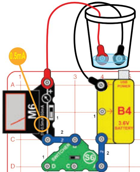
Build the circuit, set the meter (M6) to the 0.5mA setting, and set the switcher (S6) to the right position. Add about 1/4 inch of water to a cup or bowl. Connect the jumper wires to the circuit as shown and place the loose ends in the water, make sure the metal parts aren't touching each other. Measure the current through the water.
