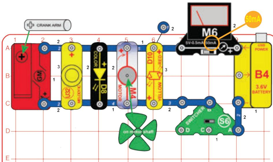
Move the meter to the new location shown and set the meter (M6) to the 50mA setting. Set the switcher (S6) to the right position and see how high the current is when the battery is running all these devices.
