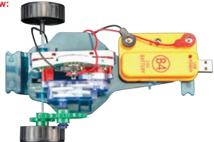
Build the circuit as shown, initially setting the switcher (S6) to the middle setting. Mount the 1.75" gear on the geared motor (GM) with the rubber rings to keep it from sliding out of position, place it on the mini car frame, and connect the battery (B4), switcher (S6) and red & black jumper wires as shown. Use the switcher to make the mini car go forward, backward-turning, or stop.
