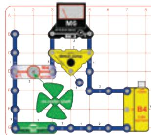
Build the circuit and set the meter (M6) to the 5V setting. Push the switch (S2); the meter measures the voltage across the motor. The voltage increases as the motor speeds up.
