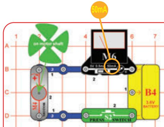
Build the circuit shown. Set the meter (M6) to the 50mA setting and place the wind fan on the motor (M4). Push the press switch (S2) and watch the current on the meter as the motor speeds up.
