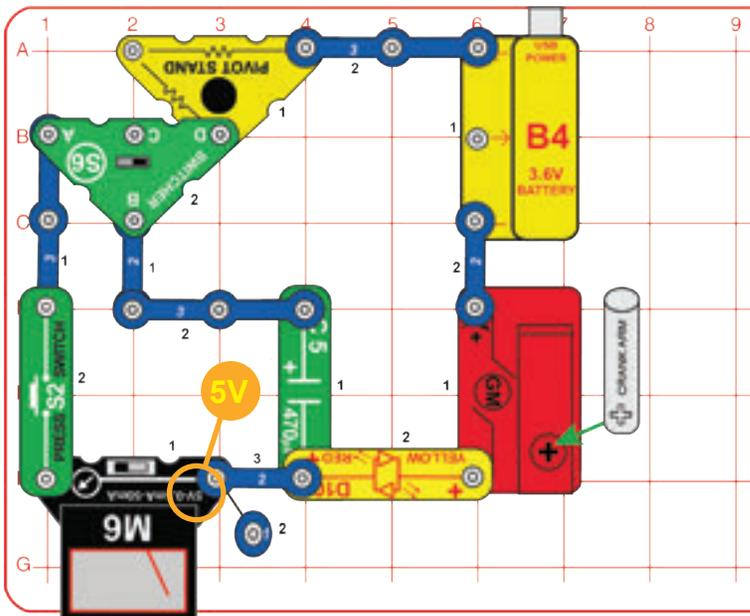
Modify the circuit to include the press switch (S2), as shown. With the switcher (S6) in the right position, turn the crank arm until the LED (D10) no longer produces light. When the capacitor is fully charged, the current is blocked and the light cannot turn on.
