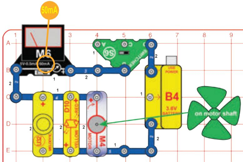
Build the circuit shown. Set the meter to the 50mA setting. Set the switcher (S6) to the right position. The battery operates the melody IC (U32), LED (D10), and motor (M4), just like batteries operate stuff in your home. The meter shows how much current is used to operate them; the more current is used, the faster the battery will run out.
