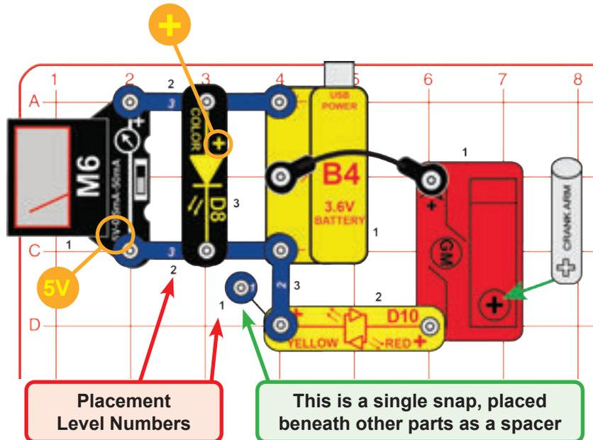
Build the circuit shown here, set the meter (M6) to the 5V setting, and place the crank arm on the geared motor (GM). The meter will measure about 3.6V if the battery is charged up.
