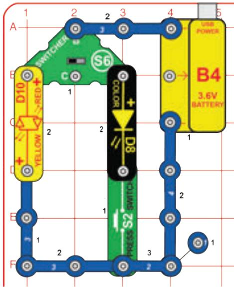
Build the circuit shown. The switcher (S6) and press switch (S2) control the lights.
