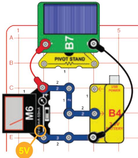
Angle adjustment to light source, measuring charge current:
