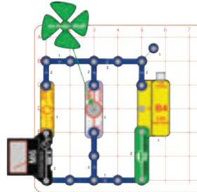
Build the circuit and set the meter (M6) to the 50mA setting. Push the switch (S2); the meter measures the current from the battery (B4). Let the fan get to full speed.
