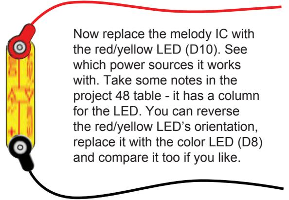
Now replace the melody IC with the red/yellow LED (D10). See which power sources it works with. Take some notes in the project 48 table - it has a column for the LED. You can reverse the red/yellow LED's orientation, replace it with the color LED (D8) and compare it too if you like.
