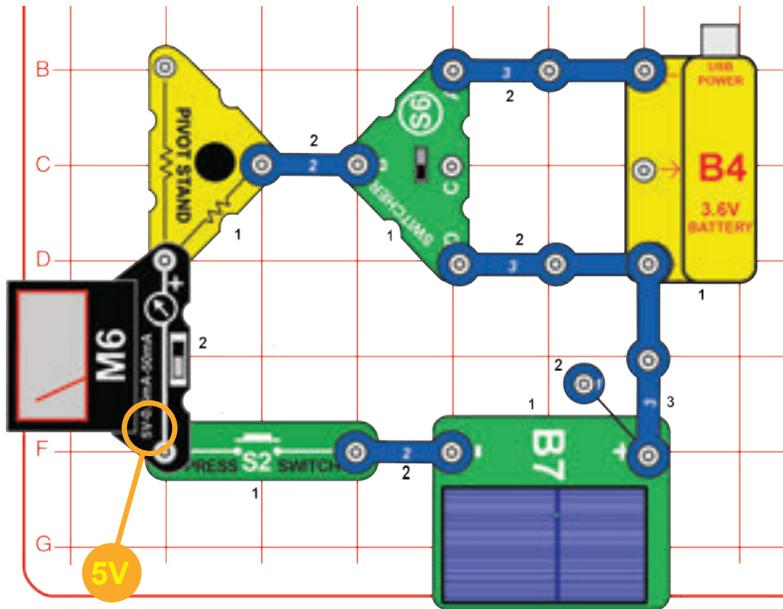
Build the circuit shown. Place the solar cell (B7) in sunlight or close to an incandescent lamp. Set the meter to the 5V setting, but double the reading it shows, since a resistor in the pivot stand converts the scale to 10V. Push the press switch (S2). If the switcher (S6) is set to the upper position, then the meter shows the combined battery (B4) and solar cell (B7) voltage. If it is set to the lower position, then the meter shows only the solar cell voltage.
