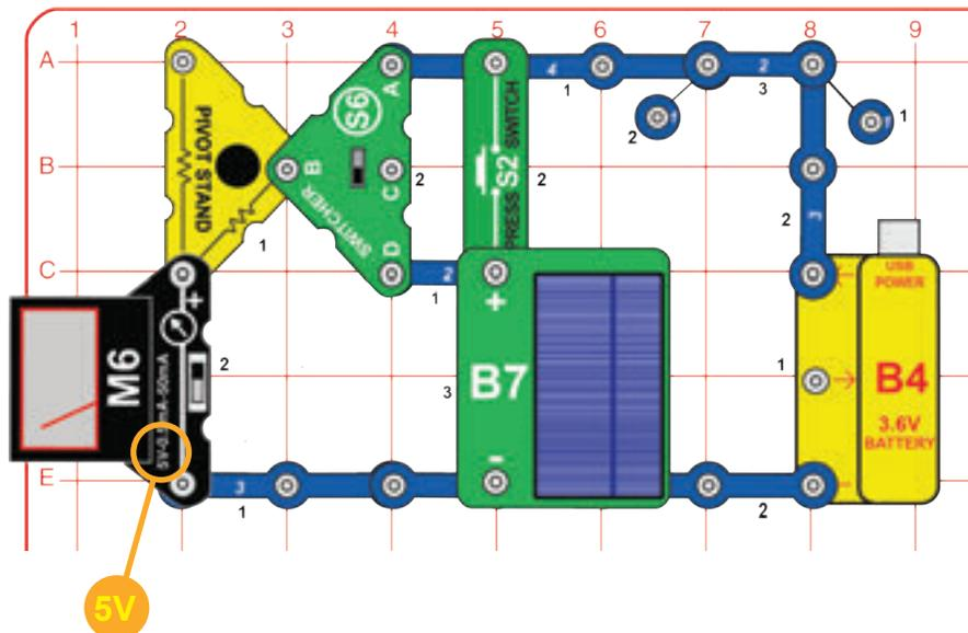
Build the circuit shown. Place the solar cell (B7) in sunlight or close to an incandescent lamp. Set the meter to the 5V setting, but double the reading it shows, since a resistor in the pivot stand converts the scale to 10V. If the switcher (S6) is set to the upper position, then the meter shows the battery (B4) voltage. If it is set to the lower position, then the meter shows the solar cell (B7) voltage.
