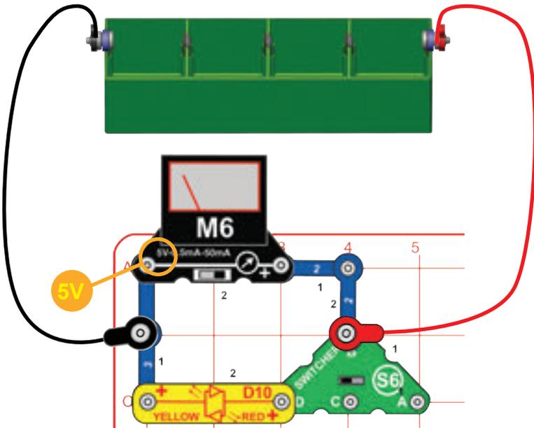
Connect the liquid energy source to the circuit shown here. Fill the compartments with water. Set the switcher (S6) to the left position. Set the meter (M6) to the 5V setting to see the voltage produced. The red/yellow LED (D10) may be dimly lit, depending on your local water supply. If you set the switcher to the right position, the voltage may be higher since the water is not trying to light the LED.
