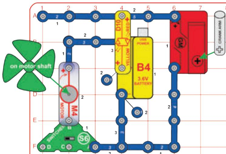
Set the switcher (S6) to the left position and turn the crank arm on the geared motor (GM). The LED (D10) lights when the crank is charging the battery (B4).
