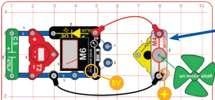
Build the circuit shown. Set the meter to the 5V setting. Blow on the fan or place it in a strong wind (either outside or near an electric fan). The meter (M6) measures how much voltage your “windmill” produces. You may need to give the fan a push to get it started.
