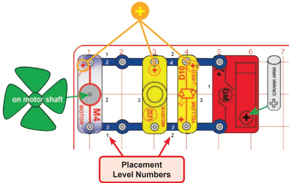
Build the circuit shown by placing all the parts with a black 1 next to them on the clear plastic base grid first. Then, assemble parts marked with a 2. Be sure to place the parts with their (+) side oriented as shown. Place the wind fan on the motor (M4) shaft, and the crank arm on the geared motor (GM). Turn the crank arm in both directions to make things happen.
