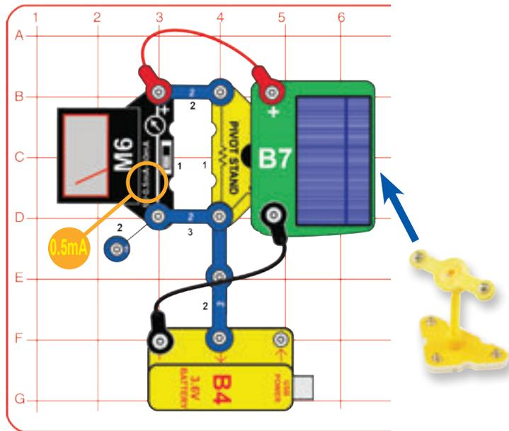
Assemble the pivot, mount the solar cell (B7) on it, and place it in the circuit as shown. Connect the solar cell to the circuit using the red and black jumper wires. Place the solar cell in sunlight or near an incandescent light bulb. The solar cell is charging the battery and the meter is measuring the current.
