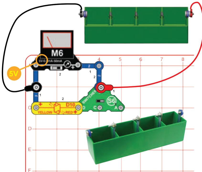
Assemble the liquid energy source using the instructions on page 4. Build the circuit and connect the red & black jumper wires; the red wire goes to the copper electrode. Set the meter (M6) to the 5V setting. Fill the compartments with cola soda (other soda flavors and lemon, tomato, or grapefruit juice also work). Set the switcher (S6) to the right position. The meter shows the voltage produced.
