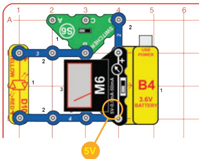
Build the circuit and set the meter (M6) to the 5V setting. Set the switch (S6) to the right position and watch the voltage on the meter for a while as the battery runs the red/yellow LED (D10). How quickly does the voltage drop?
