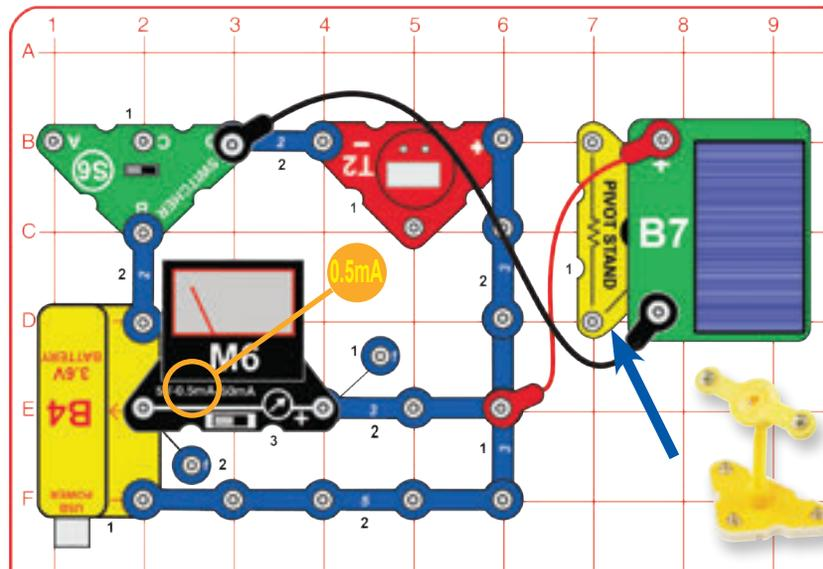
Assemble the pivot, mount the solar cell (B7) on it, and place it next to the circuit as shown. Connect the solar cell to the circuit using the red and black jumper wires. Set the meter to the 0.5mA setting. Set the Switcher switcher (S6) to the left position. Place the circuit so the solar cell is in bright sunlight or close to an incandescent light bulb. The display on the clock (T2) should be on.
