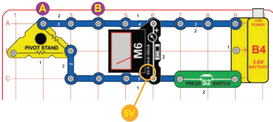
Set the meter (M6) to the 5V setting and push the press switch (S2). Read the voltage on the meter.
