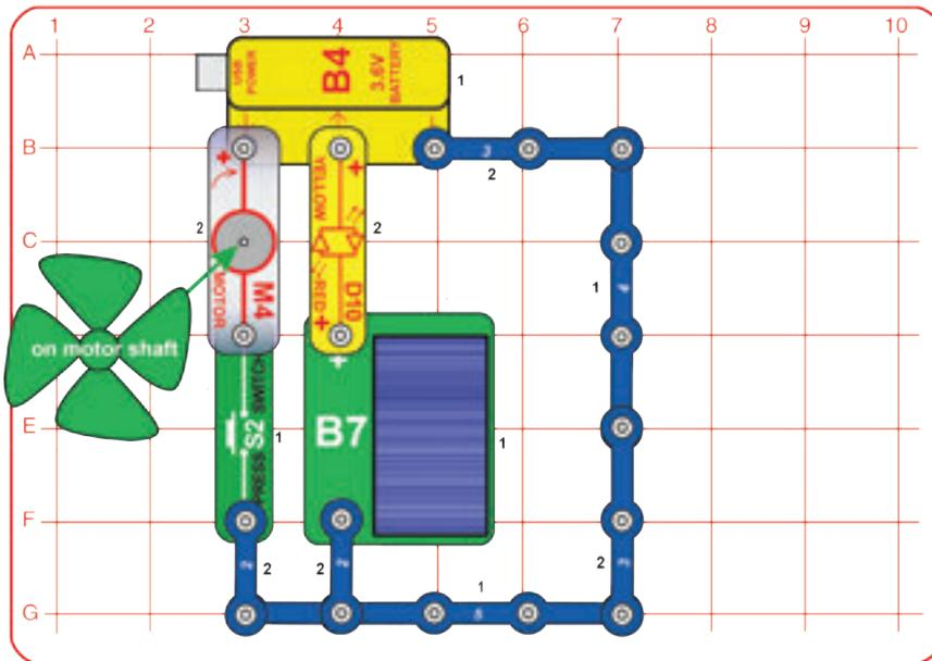
In this project you'll convert one form of energy to another. Place the solar cell in sunlight or about 12 inches from an incandescent light bulb of 60W or more. Adjust the light on the solar cell to make the red/yellow LED (D10) brightest. The solar cell converts light energy into electrical that lights the LED and charges the battery (B4).
