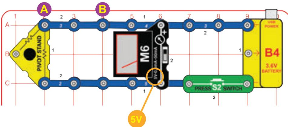
Modify the preceding circuit to be this one, which connects to a different resistor in the pivot stand. Set the meter (M6) to the 5V setting and push the press switch (S2). Read the voltage on the meter.
