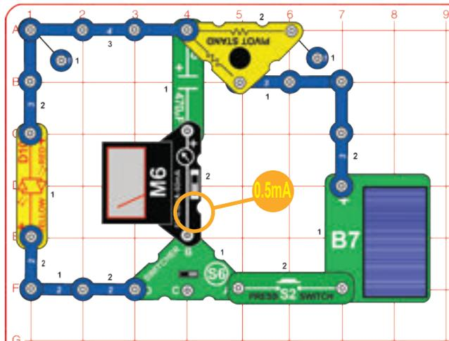
Build the circuit shown. Set the meter (M6) to the 0.5mA setting. Set the switcher (S6) to the right position, place the solar cell (B7) in sunlight or near an incandescent lamp, and push the press switch (S2). The solar cell slowly charges up the 470mF capacitor (C5), and the meter shows the current.
