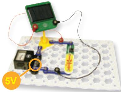
Assemble the pivot, mount the solar cell (B7) on it, and place it in the circuit as shown. Place all the parts with a black 1 next to them on the clear plastic base grid first, then parts marked with a 2. The red/ yellow LED (D10) may be connected in either direction.
