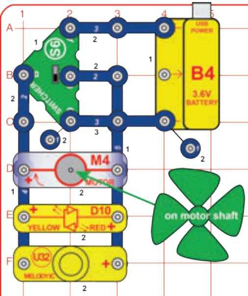
Modify the preceding circuit to be this one. Use the switcher (S6) to control light, sound, and motion. The melody IC (U32) only works in one direction.
