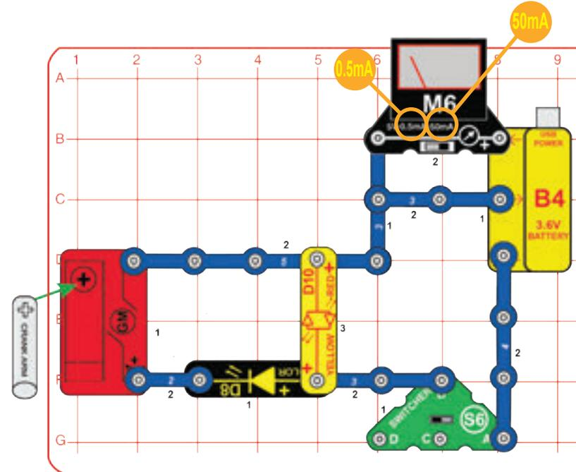
Build the circuit by setting up the parts as shown. Set the meter (M6) to the 0.5mA or 50mA setting. Set the switch (S6) to the right position to connect the rechargeable battery (B4) to the red/yellow LED (D10). If the battery is charged, the LED will light and the meter will show that an electric current is flowing out of the battery. The 0.5mA meter scale will show a high current while the 50mA scale may show little or no current.
