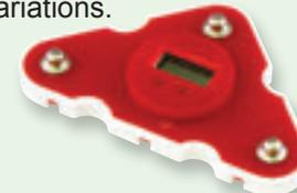
The **clock (T2)** contains a small crystal. When a crystal is struck by an electronic pulse, it vibrates. A microelectronic circuit makes the pulse and measures the vibration rate. The vibration rate is used as a time standard, from which minutes, hours, and the date are calculated.
