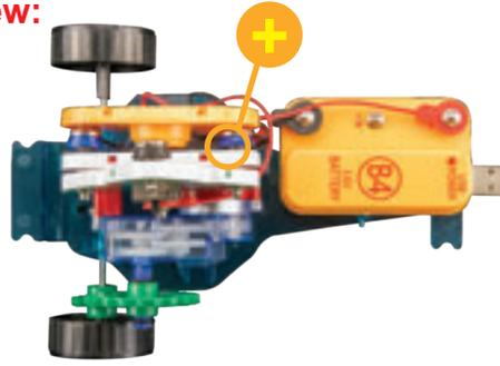
Use the project 34 circuit but add the melody IC (U32) using two 1-snap wires, as shown. A tune plays when the car moves backward. You can reverse the orientation of the melody IC to make the sound play when the car moves forward.
