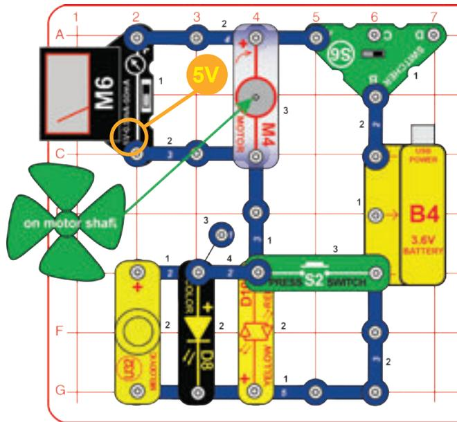
Build the circuit and set the meter (M6) to the 5V setting. Place the wind fan on the motor (M4). Set the switcher (S2) to the left position. The LEDs (D8 & D10) light, the melody IC (U32) makes sound, the fan spins, and the meter shows the voltage across the motor. You may need to give the fan a push to get it started. The voltage produced by the battery is split between the motor and the LEDs and melody IC.
