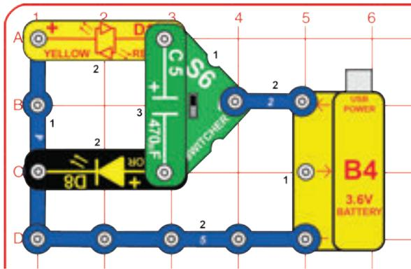
Set the switcher (S6) to the top or bottom position. Watch as one LED fades out after a few seconds, then set the switcher to the other side. Do this several times.
