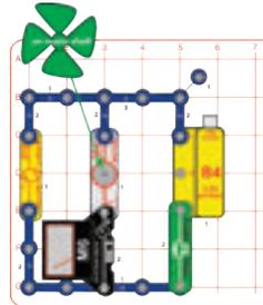
The current from the battery splits up between the LED and the motor. If you add up the current you measured through the LED and motor (Parts B & C), it should be the same as the current you measured from the battery. (Your result may be a little different, because M6 is a simple meter with low accuracy.)
