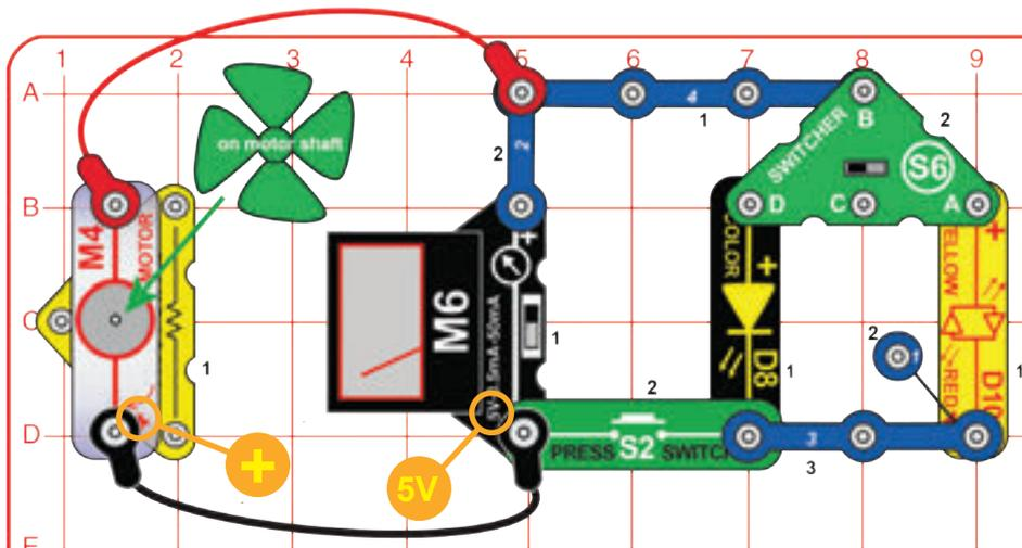
Build the circuit shown. Set the meter to the 5V setting, and the switcher (S6) to the left or right position. Blow on the fan or place it in a strong wind (either outside or near an electric fan). The meter measures how much voltage your “windmill” produces. You may need to give the fan a push to get it started.
