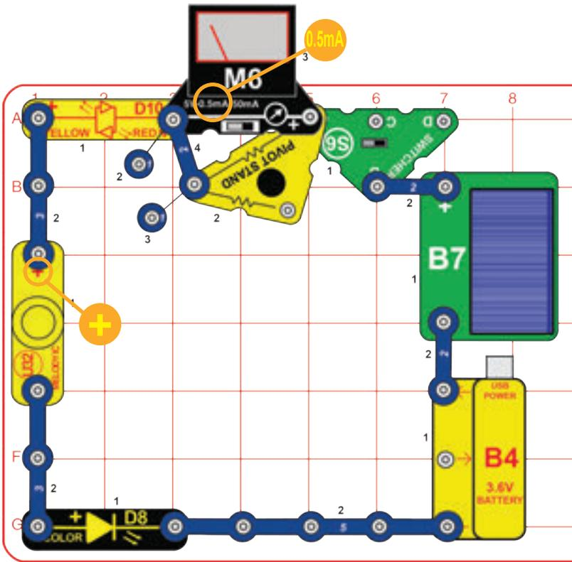
Build the circuit; it has the parts arranged in a loop. Set the meter (M6) to the 0.5mA setting. Set the switcher (S6) to the left position. Place the solar cell (B7) in bright sunlight or near an incandescent lamp. If the light is bright enough, the meter will show a current, the LEDs (D8 & D10) will light, and the melody IC (U32) will make a little noise.
