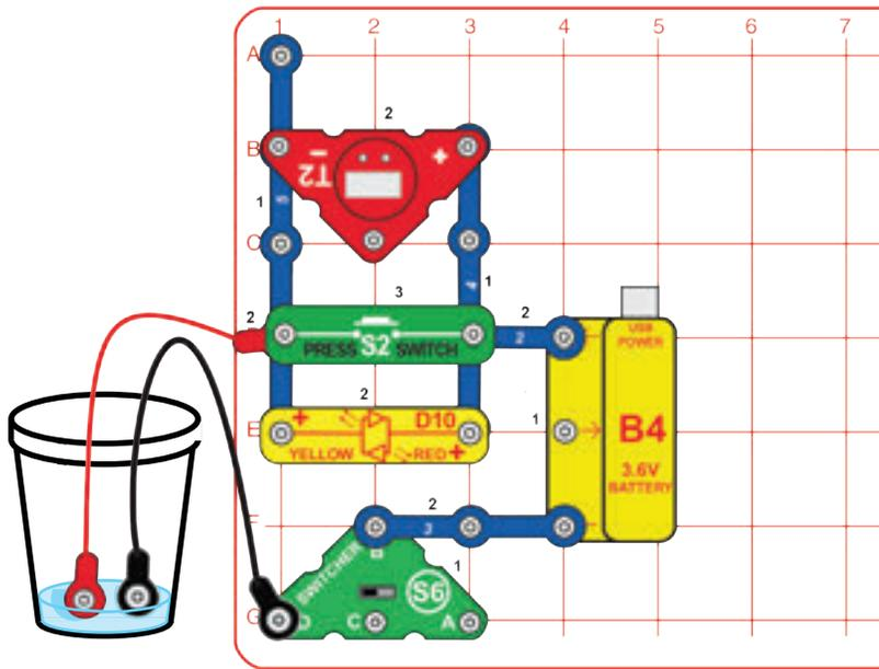
Set the switcher (S6) to the left position. Place the loose ends of the red & black jumper wires into a cup of water without the metal parts touching. The LED (D10) should light dimly and the clock (T2) should run, but it depends on your local water supply. Add salt to the water if they are off or dim to make them brighter.
