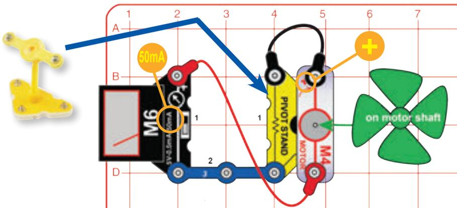
Build the circuit as shown, with the motor (M6) on the pivot and the wind fan on the motor. Set the meter (M6) to the 50mA setting. Blow on the fan or place it in a strong wind.
