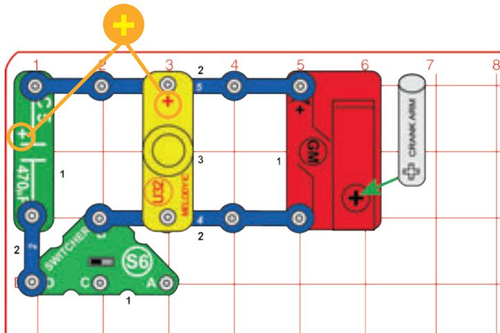
Turn the crank arm on the geared motor (GM) clockwise. The melody IC (U32) makes noise. Set the switcher (S6) to the left position to make the sound a little louder.
