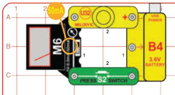
Build the circuit, set the meter (M6) to the 50mA setting. Push the switch (S2) to play a tune on the melody IC (U32), while the meter measures the current through it.
