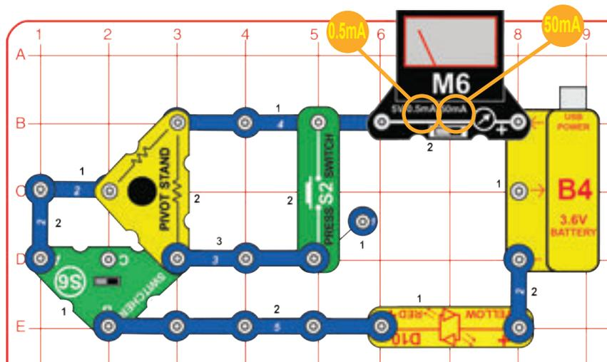
Build the circuit, set the switcher (S6) to the left position, and set the meter (M6) to the 0.5mA setting. This circuit has the red/yellow LED (D10) in series with a 10KΩ resistor in the pivot stand. 10KΩ is a high resistance, so the meter measures a small current and the LED is dimly lit. It is easier to see the LED if you take the circuit into a dark room. If the LED does not light at all then the battery needs to be recharged.
