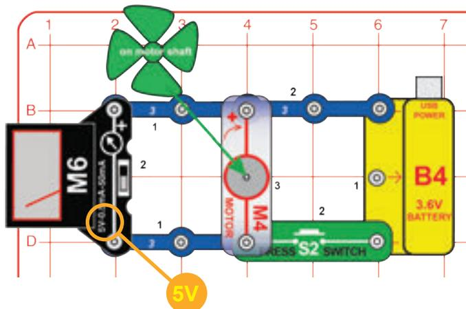
Modify the preceding circuit into this one. Set the meter (M6) to the 5V setting and place the wind fan on the motor (M4). Push and release the press switch (S2) and watch the voltage on the meter as the motor speeds up and slows down.
