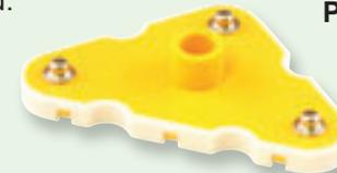
The pivot stand contains two resistors, 47W and 10KW. **Resistors** "resist" the flow of electricity and are used to control or limit the electricity in a circuit. Materials like metal have very low resistance (<1W), while materials like paper, plastic, and air have near-infinite resistance. Increasing circuit resistance reduces the flow of electricity.
