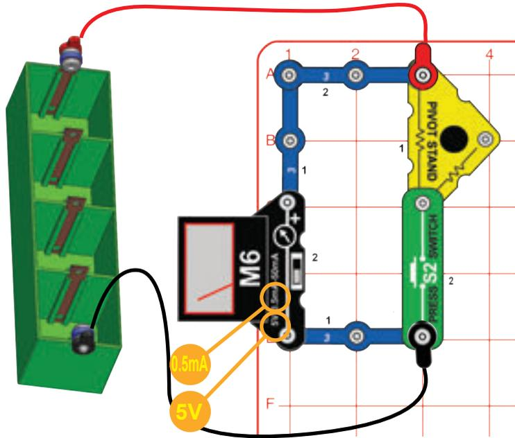
Assemble the liquid energy source using the instructions on page 4. Build the circuit and connect the red & black jumper wires; the red wire goes to the copper electrode. Set the meter (M6) to the 5V setting. Fill the compartments with water. The meter shows the voltage produced, if any.
