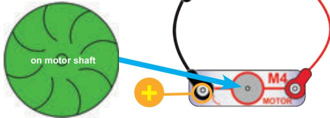
Place the water wheel on the motor (M4) and connect it to the meter (M6), as shown. Set the meter to the 5V or 50mA setting. Hold the motor under a water faucet so the water wheel will “catch” the water as it falls. See how much voltage and current you can produce.
