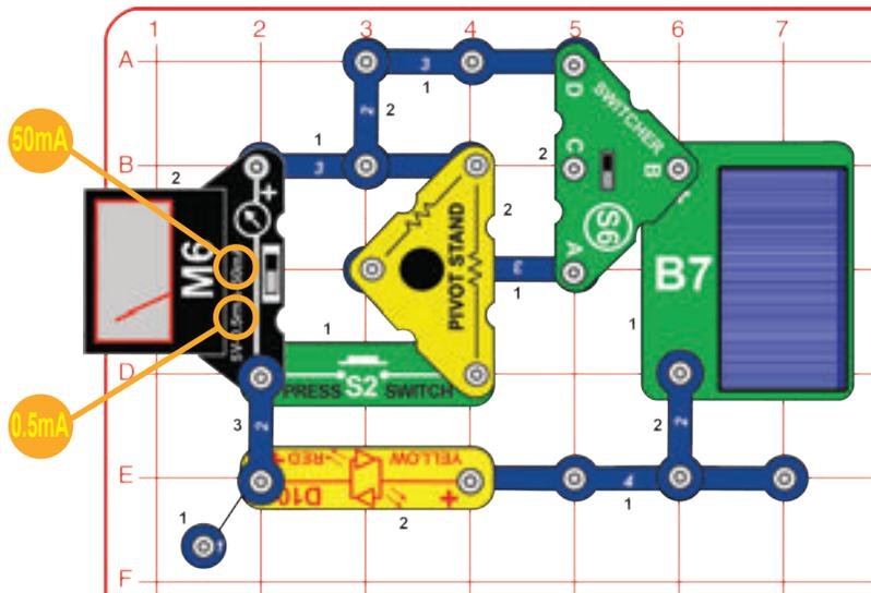
Build the circuit shown. This circuit measures current using several scales on the meter (M6). Set the switcher (S6) to the top position. Place the solar cell (B7) in sunlight or near an incandescent lamp, and vary the light on it. Use the 0.5mA or 50mA settings on the meter to measure the current through the LED (D10).
