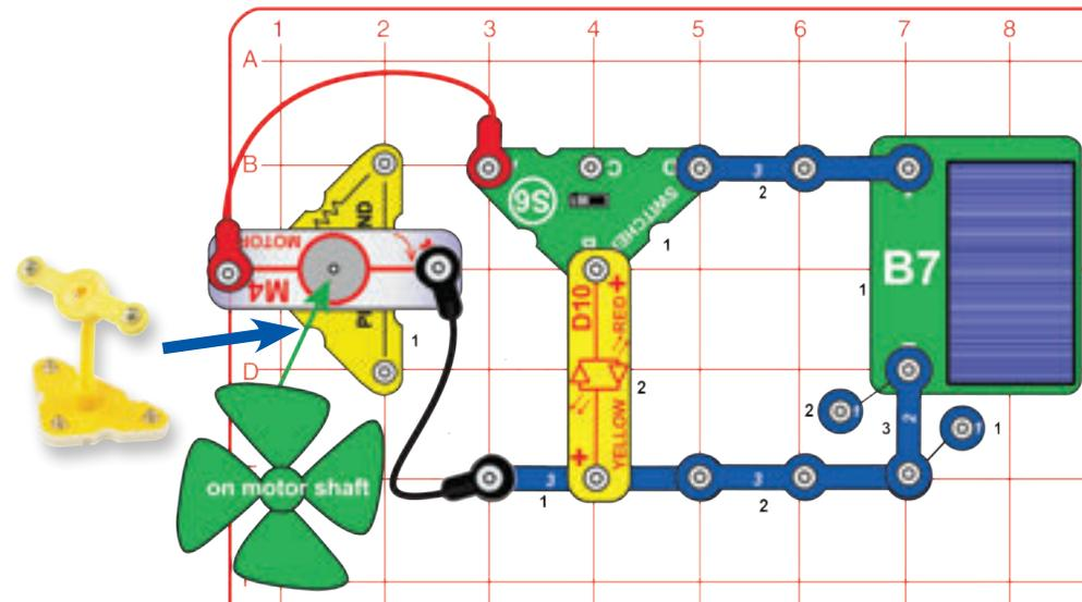
Build the circuit shown, with the motor mounted on the pivot stand like a windmill. Use either sunlight or wind power to run the red/yellow LED (D10). Set the switcher (S6) to the left to use wind power, or to the right to use solar power.
