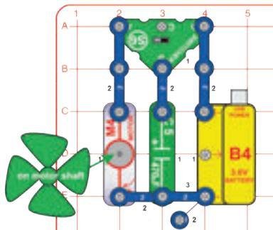
Sometimes motors under a load are difficult to get started. A capacitor can be used to give the motor a little kick. In this project setting the switcher (S6) to the right will charge the 470mF capacitor (C5), then moving it to the left will give the motor a little kick. Since no other power is applied, the motor will not go very far on the small amount of power stored in the capacitor. This is still a good way to get a motor started as power is supplied.
