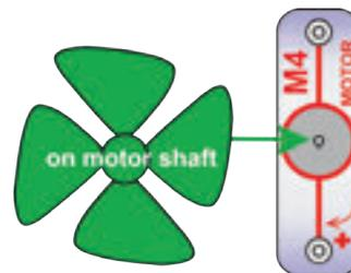
In the preceding circuit, replace the color LED (D8) with the motor (M4, in either direction) and place the wind fan on it. Now press the switch and watch how the voltage changes as the solar cell runs the fan. Depending on your light source, the fan may need a push to get started or may not work at all.
