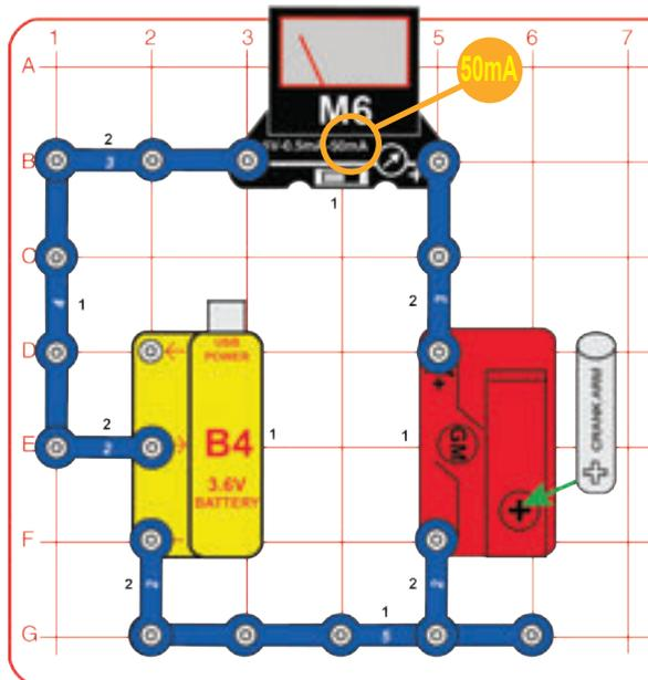
Build the circuit and set the meter (M6) to the 50mA setting. Turn the crank arm on the geared motor (GM) clockwise to charge the battery (B4), the meter measures the current. The battery will be more difficult to charge when it is near full charge.
