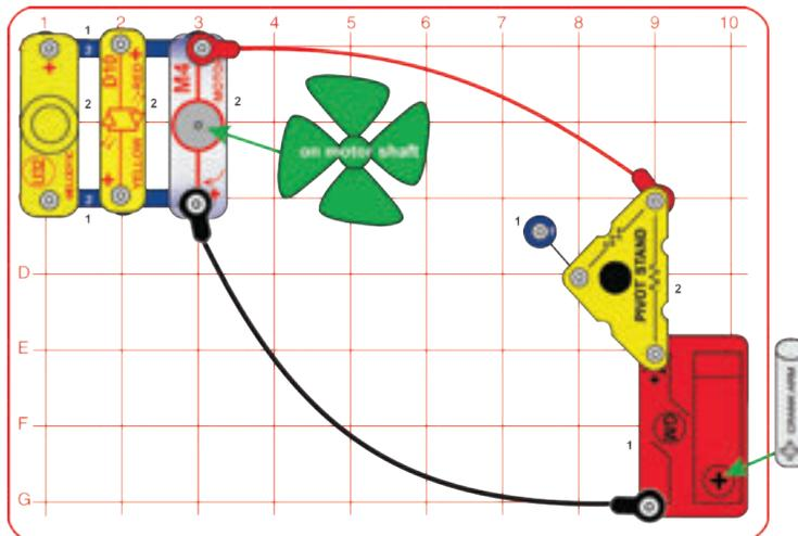
Turn the crank arm on the geared motor (GM) clockwise to run the motor (M4) and fan, red/yellow LED (D10), and melody IC (U32) or turn it backwards to run just the motor and LED.
