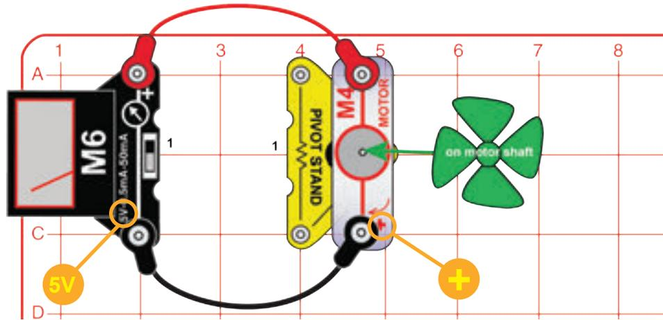
Assemble the pivot stand, mount the wind fan on the motor (M4), mount the motor on the pivot, place the pivot on the base grid and connect it to the meter (M6) using the red and black jumper wires. Set the meter to the 5V setting.
