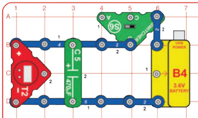
Build the circuit, and set the switcher (S6) to the right position to turn on the clock. If you turn off the switch or disconnect the power source (the B4 battery), the clock will still work for a while. The 470mF capacitor (C5) stores enough electricity to run the clock for a while during power disruptions. If you remove the capacitor, the clock will turn off when you turn off the switch.
