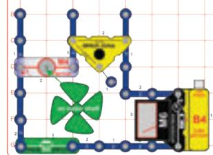
Part C: Move the meter so it is directly across the battery (B4). Push the switch to measure the voltage produced by the battery.
