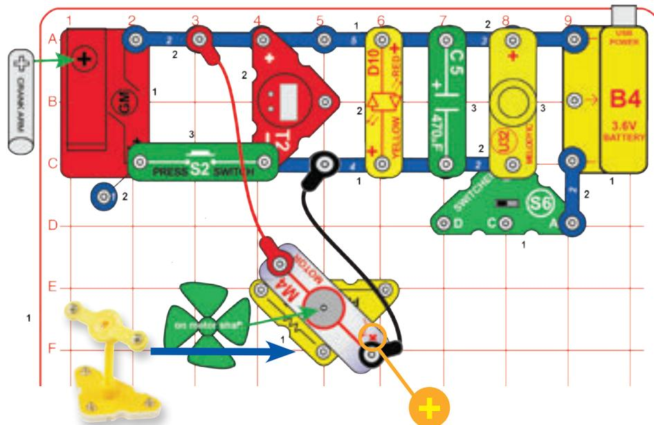
Make sure the battery is charged up (see project 3). Build the circuit with the motor and fan on the pivot stand, and connect the jumper wires as shown. Set the switcher (S6) to the right position to turn on the circuit. The battery runs the clock display (T2), melody IC (U32), red/yellow LED (D10), and windmill (M4). Push the press switch (S2) and the crank arm on the geared motor (GM) will also spin.
