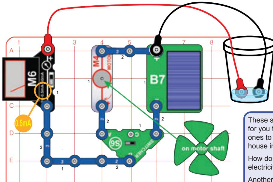
Build the circuit, place the wind fan on the motor (M4), and set the meter (M6) to the 0.5mA scale. Place the circuit so wind is blowing on the fan or sunlight is shining on the solar cell (B7). Set the switcher (S6) to the left position if you have wind or to the right position if you have sunlight. Connect the jumper wires to the circuit and place the other ends in a cup of water, make sure the metal parts aren't touching each other.
