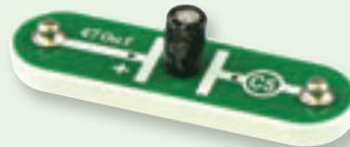
The **470mF capacitor (C5)** can store electrical pressure (voltage) for periods of time. This storage ability allows it to block stable voltage signals and pass changing ones. Capacitors are used for filtering and delay circuits.
