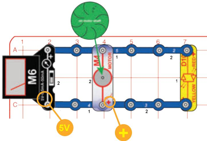
Build the circuit as shown, with the water wheel on the motor. Set the meter (M6) to the 5V setting. Blow on the water wheel, aiming the air into the “curves” on the fan. Watch the meter to see the voltage produced, and the red/yellow LED (D10) will light red.
