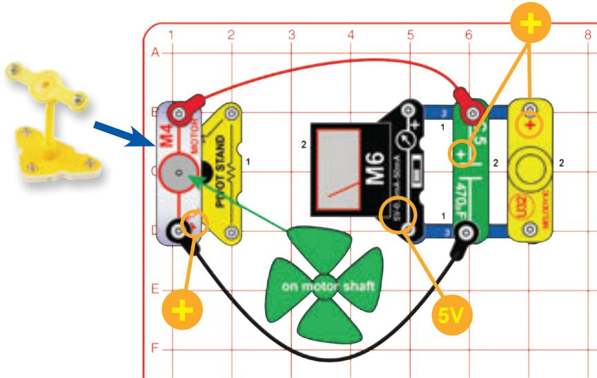
Build the circuit shown. Set the meter (M6) to the 5V setting. Blow on the fan or place it in a strong wind (either outside or near an electric fan). The meter measures how much voltage your “windmill” produces, and the melody IC (U32) makes sound from the voltage. The sound will be brief and not very loud.
