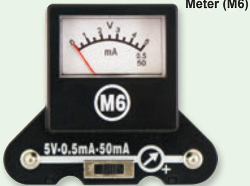
The **meter (M6)** is an important measuring device. You will use it to measure the voltage (electrical pressure) and **current** (how fast electricity is flowing) in a circuit.
