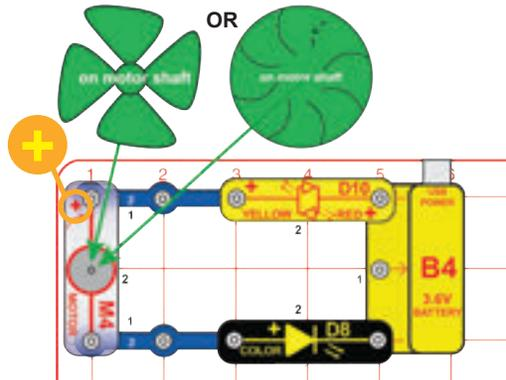
Build the circuit, and place either the wind fan or the water wheel on the motor (M4). To make the LEDs (D8 & D10) bright, blow on the wind fan from above, or blow into the “curves” of the water wheel.
