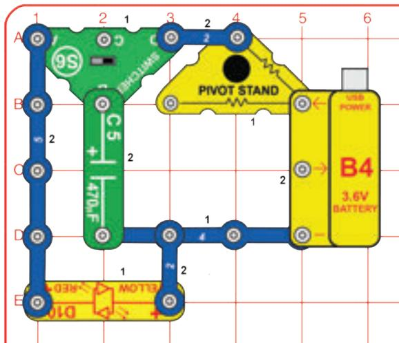
The electrons slowly trickle into the 470mF capacitor (C5) through a 10KW resistor (in the pivot stand) when the switcher (S6) is in the right position. If you wait and let the capacitor charge up it will flash nicely when you switch to the left. If you are not patient, and switch back too quickly your flash will be weak.
