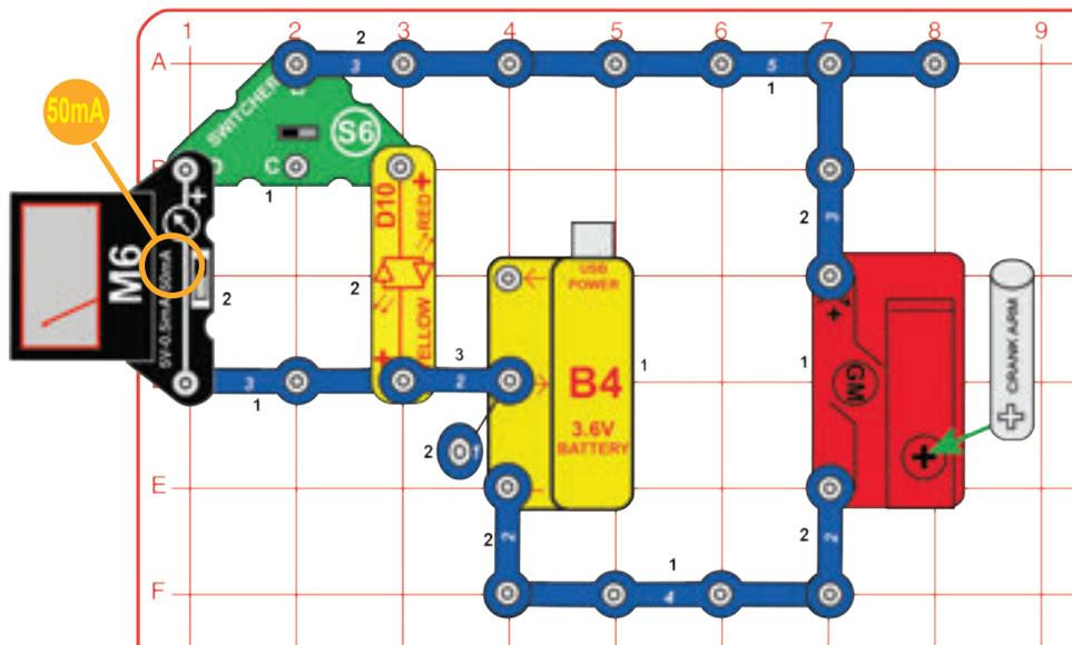
Use the crank arm to charge the battery (B4), the meter (M6) or LED (D10) show how fast you are charging it.
