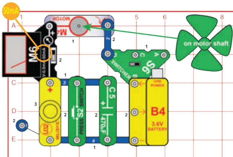
Set the meter (M6) to the 50mA setting, and set the switcher (S6) to the left position. You should hear a beeping sound from the melody IC (U32) as the meter measures the current. Spin the fan in either direction with your finger to change the sound. Push the press switch (S2) to spin the fan.
