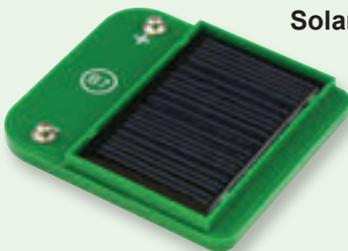
The **solar cell (B7)** contains positively and negatively charged silicon crystals,
