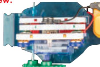
Add the red/yellow LED (D10) to the preceding circuit using two 1-snap wires and two 2-snap wires, as shown. The LED lights yellow when the car is going forward, or red when it goes backward-turning.
