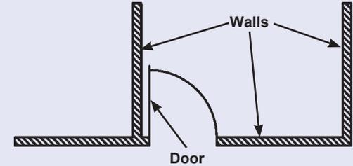
The electronics symbol for a simple switch should be thought of as a door to a circuit, which swings open when the switch is off. The “door” to the circuit is closed when the switch is on. This is shown here:
