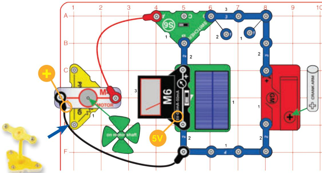
Build the circuit shown and set the meter to the 5V setting. Set the switcher to the middle position and the meter measures the voltage produced by the solar cell. Next, set the switcher to the left position and blow on the windmill to see the voltage it produces. Next, set the switcher to the right position and turn the crank arm to see the voltage it produces.
