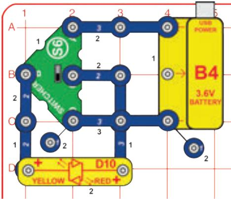
Build the circuit shown. Use the switcher (S6) to control the light.
