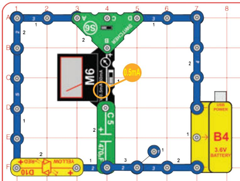
Build the circuit shown. Set the meter (M6) to the 0.5mA setting. Flip the switcher (S6) back and forth between its left and right positions to charge and discharge the 470mF capacitor (C5).
