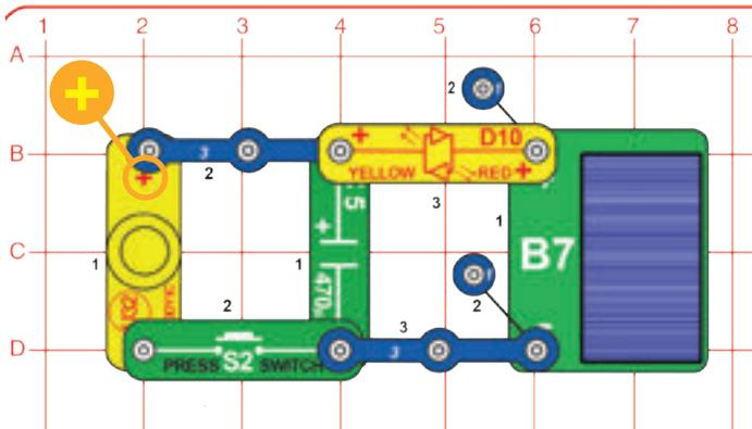
The capacitor stores energy as an electric field, similar to the magnetic field of a magnet. It can only store a small amount of energy in this way.
