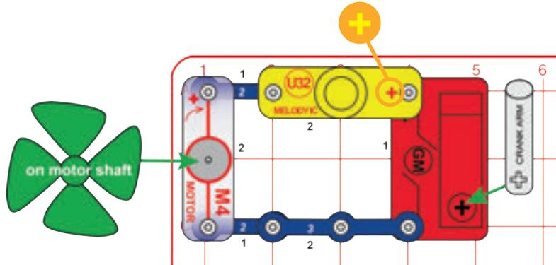
Turn the crank arm clockwise to run the fan and melody IC (U32).
