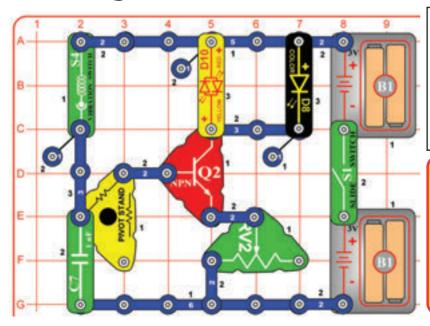
Build the circuit and turn on the slide switch (S1). Bang on the table or tap on the vibration switch (S4) and lights come on. The lights stays on for a while after the vibrations end. The lever on the adjustable resistor (RV2) controls the maximum light brightness and how long the lights stays on after vibrations end; the brighter the lights, the faster they shut off.
