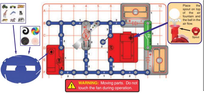
Build the circuit. Place the merry-go-round base on the geared motor (GM) shaft; if desired, insert some of the cardboard figures into the base or install one of the colored discs into it. Turn on the slide switch (S1).
