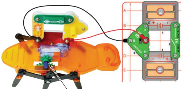
Assemble the crawler using the assembly instructions on pages 6 and 7, and build the circuit shown here. Mount the smallest gear (1.0") on the geared motor (GM) with a rubber ring to keep it from sliding out of position, and place it on the crawler frame. Mount the red/yellow bicolor LED (D10), vibration switch (S4), and pivot stand to the geared motor in the arrangement shown, and connect to the circuit on the base grid using the red & black jumper wires as shown.
