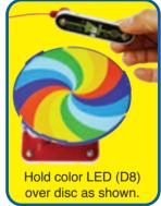
If the color LED flash rate is synchronized with the disc rotation speed, it can appear to "freeze" parts of the spinning disc pattern. Also, as different colors flash, those colors can seem to disappear.
