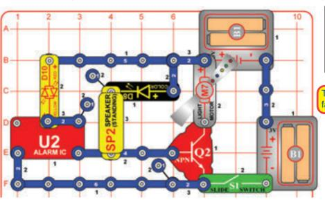
Build the circuit and turn on the slide switch (S1). The light motor (M7) spins in short bursts, synchronized with a machine qun-like sound.
