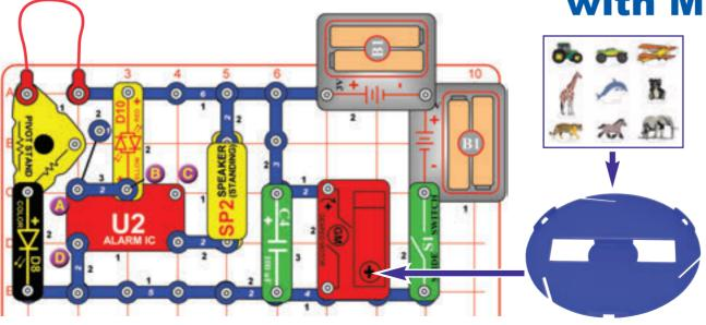
Insert some of the cardboard figures into the 3 slots on the edge of the merry-goround base (the figures may need to be punched out of a cardboard sheet). Build this circuit and mount the merry-goround base onto the shaft on the geared motor (GM).
