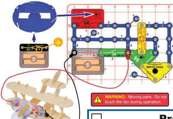
Assemble the airplane using the instructions on page 5, install the light motor (M7) into the front of it, build the circuit shown here, and connect the red & black jumper wires to the light motor (red to "+"). Place the airplane on a smooth surface and spread out the jumper wires and be sure they will not interfere with the fan on the light motor.
