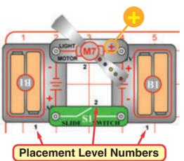
Boffin uses electronic blocks that snap onto a clear plastic grid to build different circuits. These blocks have different colors and numbers on them so that you can easily identify them.
