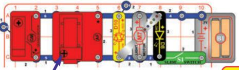
Build the circuit, but note that the air fountain (AF) is placed over the middle of the 5-snap and 6-snap wires. Place the spout on top of the air fountain and place the ball in it. Turn on the slide switch (S1).
