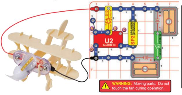
Assemble the airplane using the instructions on page 5, install the light motor (M7) into the front of it, build the circuit shown here, and connect the red & black jumper wires to the light motor (red to "+"). Spread out the jumper wires and be sure they will not interfere with the fan on the light motor.
