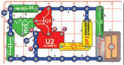
The adjustable resistor (RV2) is used here as a fixed resistor (10k $\Omega$  value), so moving its lever won't do anything.
