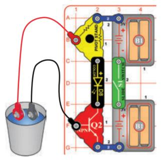
Build the circuit and turn on the switch (S1). Touch the metal in the jumper wire snaps with your fingers; the color LED (D8) should light. If the LED is dim or off, hold the metal more tightly or wet your fingers.
