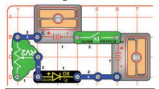
Build the circuit and turn on the slide switch (S1). Move the lever on the adjustable resistor (RV2) to vary the brightness of the light from the color LED (D8).
