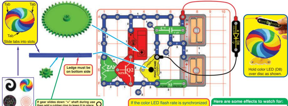
Build the circuit shown. Mount the 3.3" gear on the geared motor (GM), mount the 1.0" gear on the "+" shaped bar, place the "+" bar into the pivot stand, and then align the position of the 1.0" gear on the "+" shaft so the teeth of both gears mesh. Install one of the colored discs into the merry-go-round base. Mount the merry-goround base onto the top of the "+" shaped bar. Connect the color LED (D8) using the red & black jumper wires.
