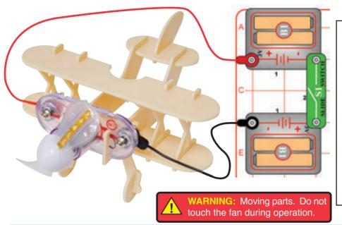
Assemble the airplane using the instructions on page 5, install the light motor (M7) into the front of it. build the circuit shown here, and connect the red & black jumper wires to the light motor (red to "+"). Spread out the jumper wires and be sure they will not interfere with the fan on the light motor.
