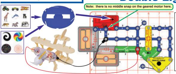
Modify the preceding circuit by removing the color LED (D8) and adding the second battery holder (B1) to the circuit as shown. Either insert some of the cardboard figures into the 3 slots on the edge of the merry-goround base, or install one of the colored discs into the base. Mount the merry-go-round base onto the shaft on the geared motor (GM). Turn on the slide switch (S1).
