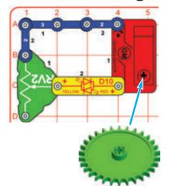
Normally, the geared motor uses electricity to create mechanical motion. This circuit uses the geared motor in reverse, to use mechanical motion (from you spinning the shaft) to create electricity (to light the LED).
