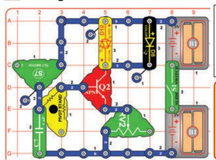
Build the circuit and turn on the slide switch (S1). Lights comes on if the circuit is moved, or tilted in some directions. The lights stay on for a while after the tilt is removed. The lever on the adjustable resistor (RV2) controls the maximum light brightness and how long the lights stay on after tilt is removed; the brighter the lights, the faster they shut off.
