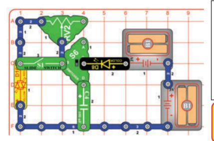
Modify the preceding circuit to match this one. Turn off the slide switch (S1); now the adjustable resistor (RV2) controls how quickly the  $100\mu F$  capacitor (C4) discharges through the red/yellow LED (D10). Setting RV2 to the left makes D10 flash brightly but briefly; setting RV2 to the right makes the LED dimmer but it stays on longer.
