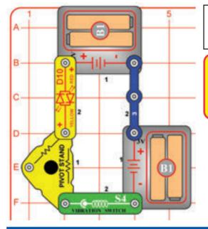
Build the circuit as shown. Tap on the vibration switch (S4) or bang on the table to make the red/yellow LED (D10) light.
