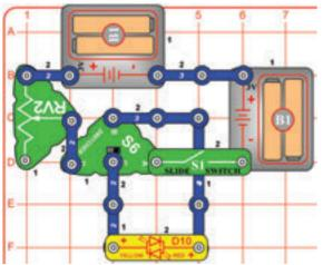
Modify the preceding circuit to match this one. With the slide switch (S1) on, use the switcher (S6) to set the color of the red/yellow bicolor LED (D10) and use the adjustable resistor (RV2) to set the brightness.
