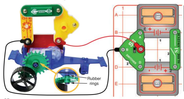
Mount the 1.75" gear on the geared motor (GM), with the rubber rings to keep it from sliding out of position, and place it on the mini car frame. Mount the red/yellow bicolor LED (D10), vibration switch (S4), and pivot stand to the geared motor in the arrangement shown, and connect to the circuit on the base grid using the red & black jumper wires as shown.
