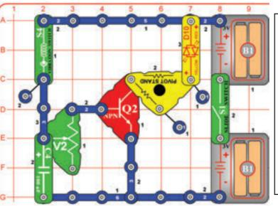
Modify the preceding circuit to be this one. Turn on the slide switch (S1). Bang on the table or tap on the vibration switch (S4) and a light comes on. The light stays on for a while after the vibrations end. The lever on the adjustable resistor (RV2) controls the maximum light brightness and how long the light stays on after vibrations end; the brighter the light, the faster it shuts off.
