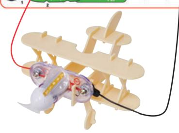
This circuit runs the air fountain (AF) at 3V instead of 6V. Now the air fountain doesn't operate at full power, but it uses less current from the batteries. The lower current here will rarely (or never) activate the fuse like it could in the preceding project, and if the fuse does activate it would only be after a much longer operating time.
