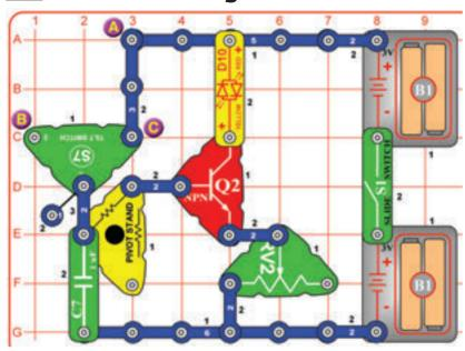
When tilt is detected, the  $1\mu F$  capacitor (C7) is charged through the tilt switch (S7). When tilt is removed, the capacitor discharges through the resistors in the pivot stand and RV2, and through the NPN transistor (Q2). The light stays on as the capacitor discharges. RV2 also limits the current through the LED (D10), and so affects the LED brightness.
