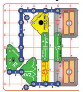
The  $100\mu F$  capacitor (C4) is like a mini rechargeable battery because it can store electricity. In this circuit, turning on S1 charges up the capacitor, which holds the electricity after S1 is turned off. Turning on S6 creates a circuit path through RV2 for the capacitor to discharge through.
