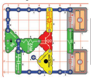
Set the switcher (S6) to the top position and turn on the slide switch (S1). The red/yellow bi-color LED (D10) is on. Now set S6 to the middle position and wait; the LED goes off after a little while. The adjustable resistor (RV2) can adjust how quickly the light goes out.
