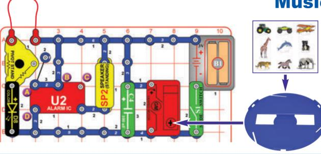
Insert some of the cardboard figures into the 3 slots on the edge of the merry-goround base (the figures may need to be punched out of a cardboard sheet). Build this circuit and mount the merry-goround base onto the shaft on the geared motor (GM).
