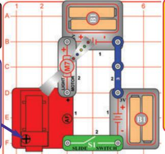
Motors need lots of electric current when they start up, then much less when their shafts are spinning at high speed (it is harder to get the shaft spinning than to keep it spinning). Compare this to riding a bicycle: you have to pedal harder to get going, then it's easy to keep going at a constant speed.
