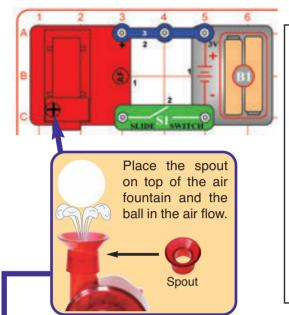
Build the circuit as shown, place the spout on the air fountain (AF), turn on the slide switch (S1), then place the ball directly in the blowing air above the air fountain. The blowing air should balance the ball, so it floats in the air and "dances". Occasionally the ball may become unstable and fall out; just place it back into the air flow.
