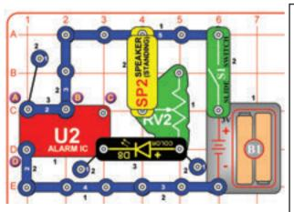
Build the circuit and turn on the slide switch (S1). Use the lever on the adjustable resistor (RV2) to change the sound volume and light brightness.
