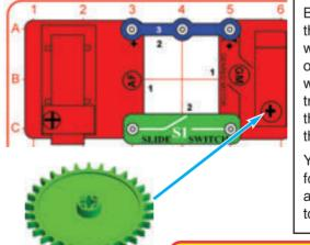
Build this circuit, and mount the 2.55" gear on the geared motor (GM). GENTLY spin the gear with your hand with the slide switch (S1) both on and off. Compare how difficult it is to turn whether the switch is on or off. You can also try this with different gears. Do not try to spin the gear with too much force or you may break the geared motor.
