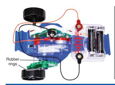
Build the circuit shown here. Mount the 1.75" gear on the geared motor (GM) with the rubber rings to keep it from sliding out of position, and place it on the mini car frame. Place the switcher (S6) directly on the geared motor, set S6 to the middle position, place a battery holder (B1) on the front of the mini car frame, connect the red jumper wire from + on B1 to C on S6, then connect black wire from — on B1 to B on S6. Be sure the jumper wires will not interfere with the gears or wheels.
