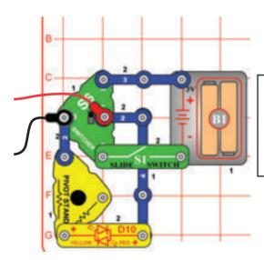
Modify the preceding circuit to include the red/yellow bicolor LED (D10), which lights yellow when the car is going forward, or red when it goes backward-turning.
