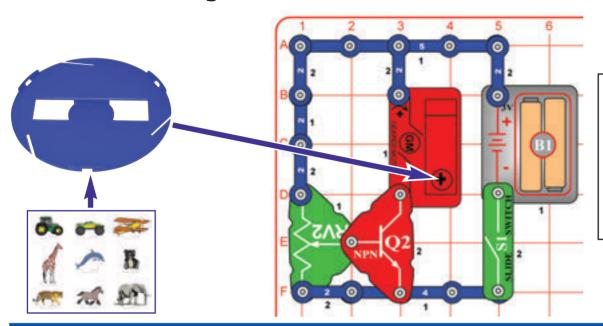
Insert some of the cardboard figures into the 3 slots on the edge of the merry-go-round base (the figures may need to be punched out of a cardboard sheet). Build this circuit and mount the merry-go-round base onto the shaft on the geared motor (GM).
