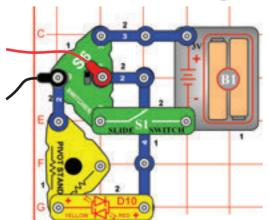
Modify the preceding circuit to include the red/yellow bicolor LED (D10), which lights yellow when the crawler is going forward, or red with it goes backward.
