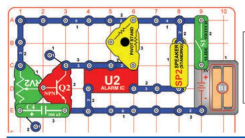
Set the adjustable resistor (RV2) to the bottom position. Turn on the slide switch (S1). A machine gun sounds for a second, then stops. Turn off the slide switch, wait a few seconds, then turn it back on to hear the machine gun sound again. Try this several times.
